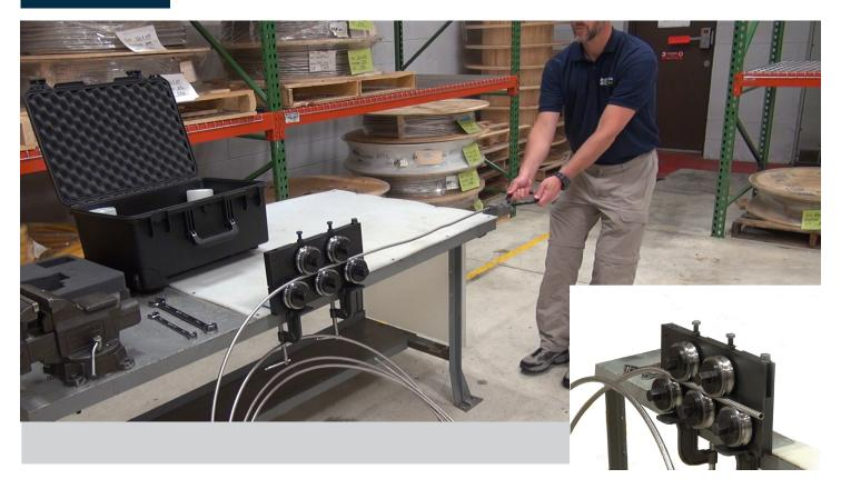
New Methods Improving Efficiency and Reducing Waste Using coiled tubing allows installers to run continuous lines of seamless tubing without fittings or welding. The tube straightener allows installers to straighten exactly what they need, reducing waste and connections.
